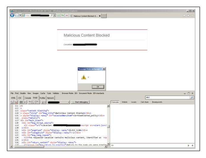
Figure 5. This universal XSS introduced by Sophos Web Intelligence defeats the Same Origin Policy, the fundamental security foundation the web is built on
